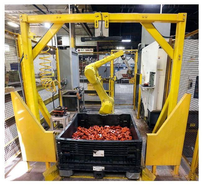
A robotic machine picks up and surfaces parts during a typical work day at M & H Valve in Anniston. Photo by Stephen Gross/The Anniston Star
