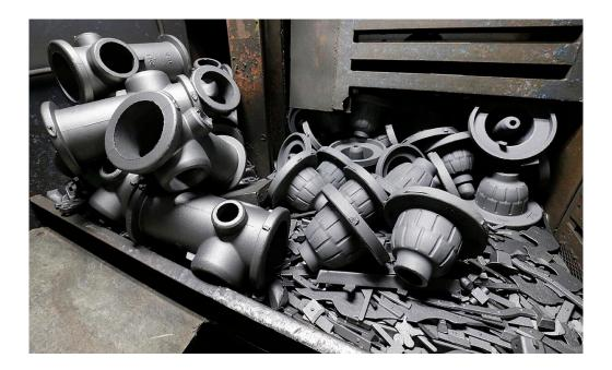
Freshly poured fire hydrant parts rest in a bin after an initial cleaning at M & H Valve in Anniston. Photo by Stephen Gross/The Anniston Star
