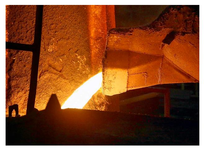
A bucket holding 6 tons of molten iron fills a hopper that feeds into fire hydrant sand molds at M & H Valve in Anniston. Photo by Stephen Gross/The Anniston Star
