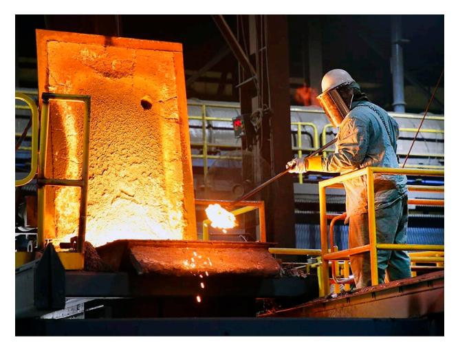
An employee pulls off slag from a hopper full of molten iron that feeds into fire hydrant sand molds at M & H Valve in Anniston. Photo by Stephen Gross/The Anniston Star
