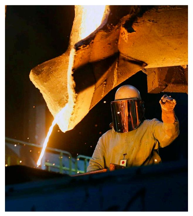
An employee guides a bucket holding 6 tons of molten iron into a hopper that feeds into fire hydrant sand molds at M & H Valve in Anniston. Photo by Stephen Gross/The Anniston Star
