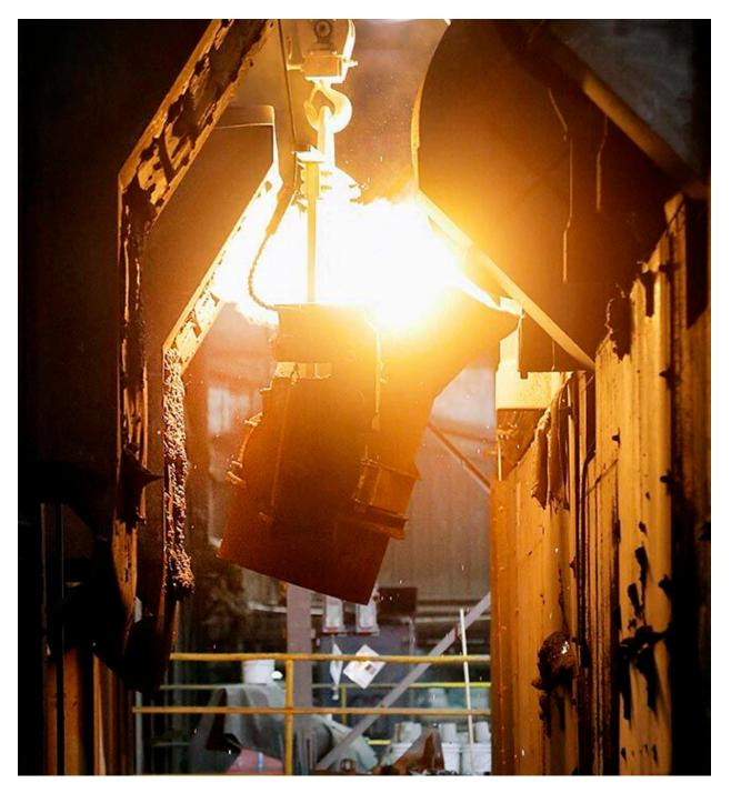
A bucket refills with 6 tons of molten iron to pour into fire hydrant sand molds at M & H Valve in Anniston. Photo by Stephen Gross/The Anniston Star
