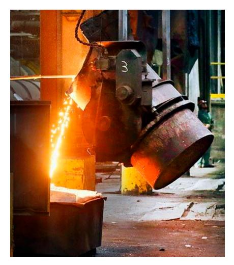
A bucket holding 6 tons of molten iron pours off slag before filling a hopper that feeds into fire hydrant sand molds at M & H Valve in Anniston. Photo by Stephen Gross/The Anniston Star
