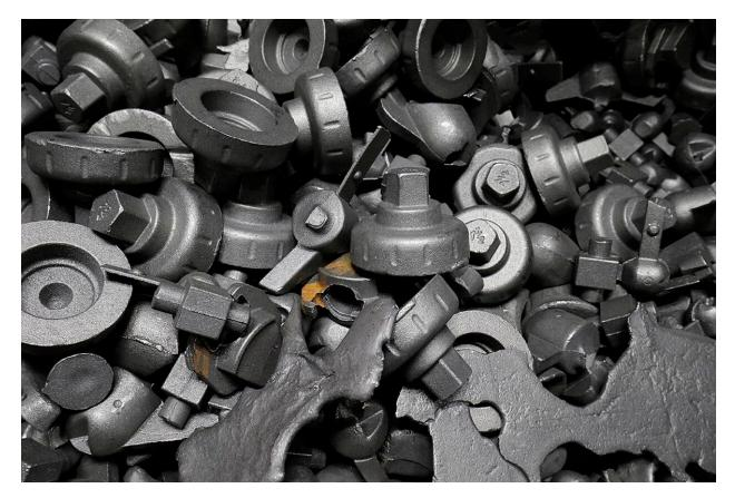
Freshly poured fire hydrant parts rest in a bin after an initial cleaning at M & H Valve in Anniston. Photo by Stephen Gross/The Anniston Star
