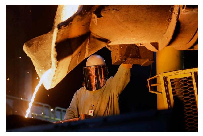
An employee guides a bucket holding 6 tons of molten iron into a hopper that feeds into fire hydrant sand molds at M & H Valve in Anniston. Photo by Stephen Gross/The Anniston Star
