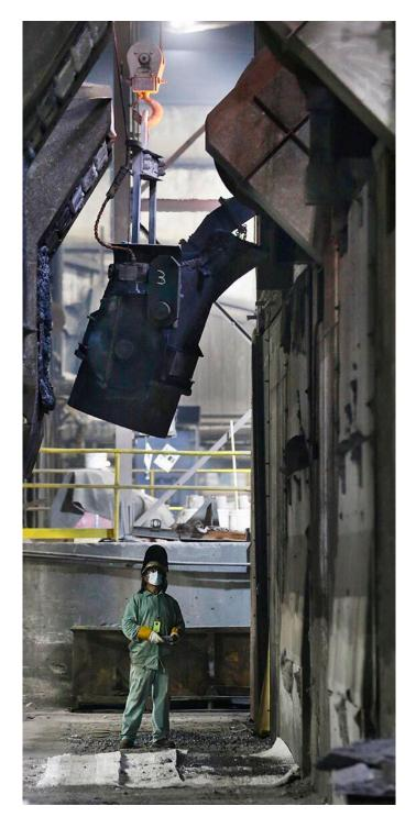
An employees remotely guides a bucket into place for refilling 6 tons of molten iron to pour into fire hydrant sand molds at M & H Valve in Anniston. Photo by Stephen Gross/The Anniston Star
