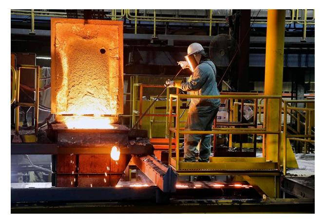
An employee pulls off slag from a hopper full of molten iron that feeds into fire hydrant sand molds at M & H Valve in Anniston. Photo by Stephen Gross/The Anniston Star
