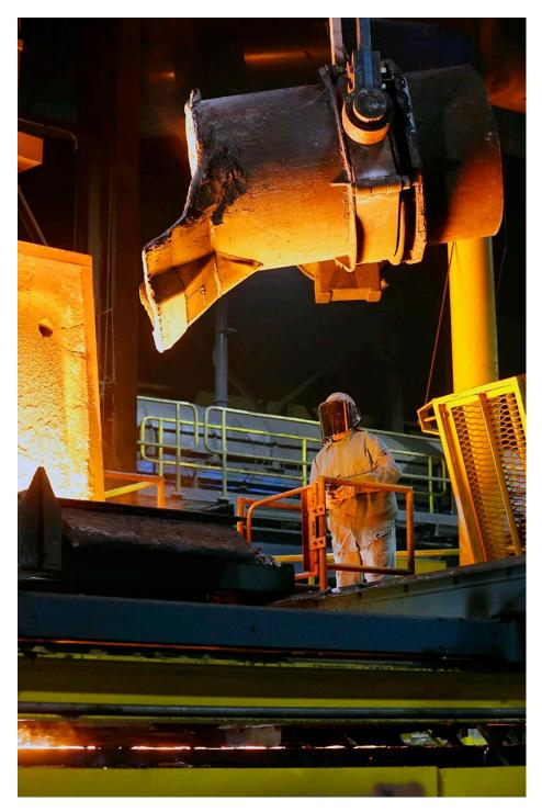
An employee guides a bucket holding 6 tons of molten iron into a hopper that feeds into fire hydrant sand molds at M & H Valve in Anniston. Photo by Stephen Gross/The Anniston Star
