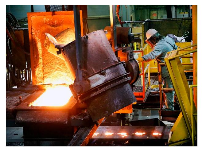
An employee guides a bucket holding 6 tons of molten iron into a hopper that feeds into fire hydrant sand molds at M & H Valve in Anniston. Photo by Stephen Gross/The Anniston Star
