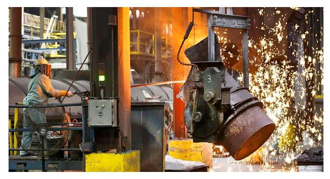
An employee guides a bucket holding 6 tons of molten iron into a hopper that feeds into fire hydrant sand molds at M & H Valve in Anniston. Photo by Stephen Gross/The Anniston Star
