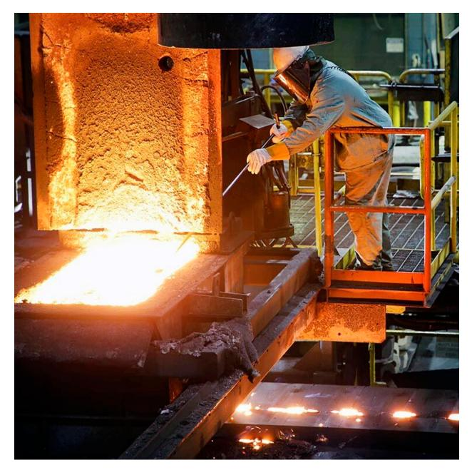
An employee pulls off slag from a hopper full of molten iron that feeds into fire hydrant sand molds at M & H Valve in Anniston. Photo by Stephen Gross/The Anniston Star
